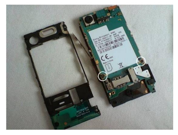
• The circuit board will now be loose but still connected by a ribbon. Again, flick the black latch over to release the ribbon.
