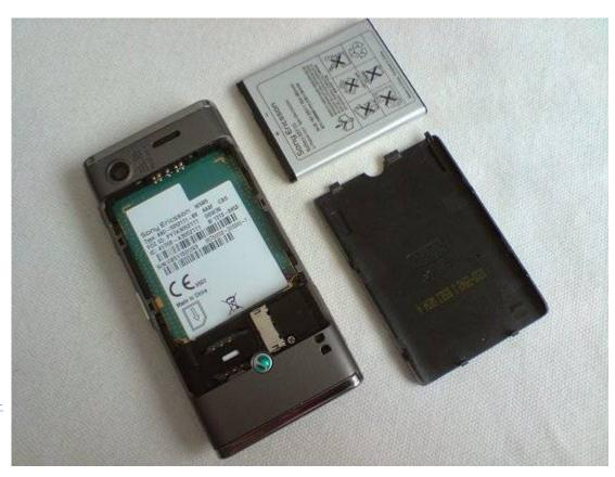
• Run something like a credit card under the metal plate at the top of the phone. It is stuck down tight with double sided tape but it will come away with a little force.
