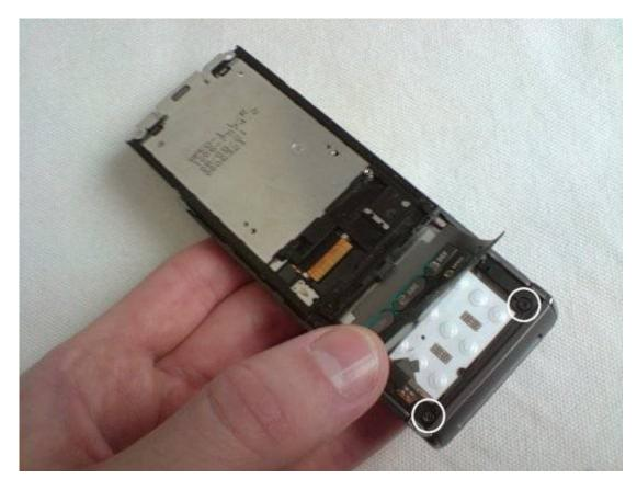
• Run your credit card around the join of the grey part of the phone to release a number of clips. Turn the phone over and release a few more clips in the battery compartment.
