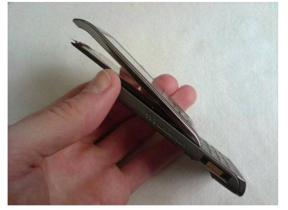
You should now have the front cover removed. Remove the small screw you can see.
