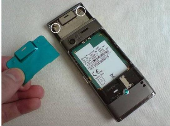
Starting near the top of the phone, run your credit card along the join of the front cover. When you have released the cover as much as shown below, slide the cover down to remove it (clips hold the cover on at the bottom which will be bent if you don't slide the cover off).
