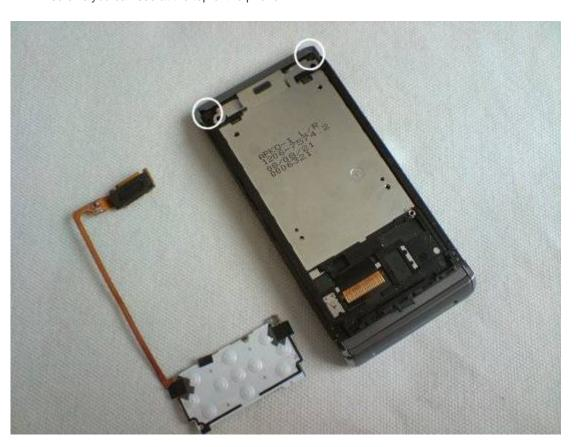
• You now need to lift the keypad up. It's stuck down lightly with double sided tape. Remove the two screws you can see.
