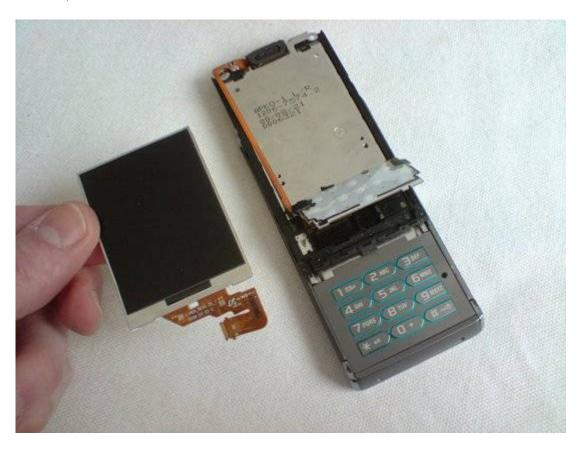
• Remove the speaker and connecting ribbon etc. It's just stuck down lightly. Remove the two screws you can see at the top of the phone.
