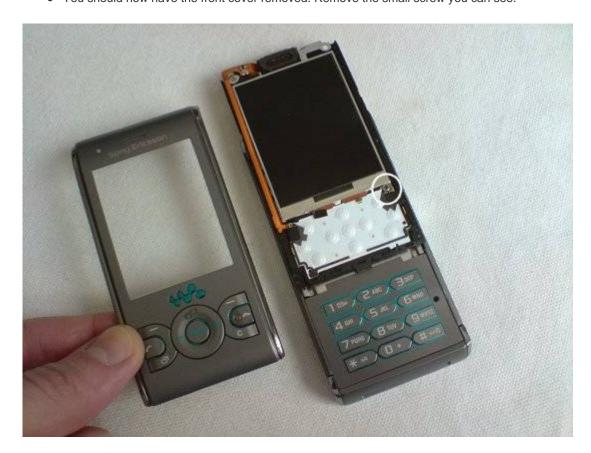
• With the slide open halfway, lift the up the part you've just removed the screw from to reveal three ribbon connectors. Each connector has a black latch which you need to flick over the release the ribbon.
