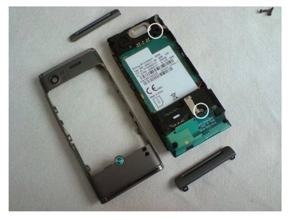
• You can now remove the battery compartment. A ribbon is stuck to the side of this and will peel away quite easily. Remove the two screws you can see.
